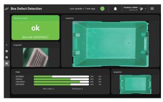
Fig. 8 Software interface of Box Defect Detection.
